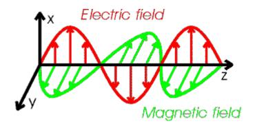
A. Light can be thought of either in terms of an oscillating magnetic field or an oscillating electric field. Light oscillating like this in a single plane (in terms of the electric field) is called
