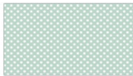
Dots —40% coverage; 1/8" dots staggered on 1/4" centers
