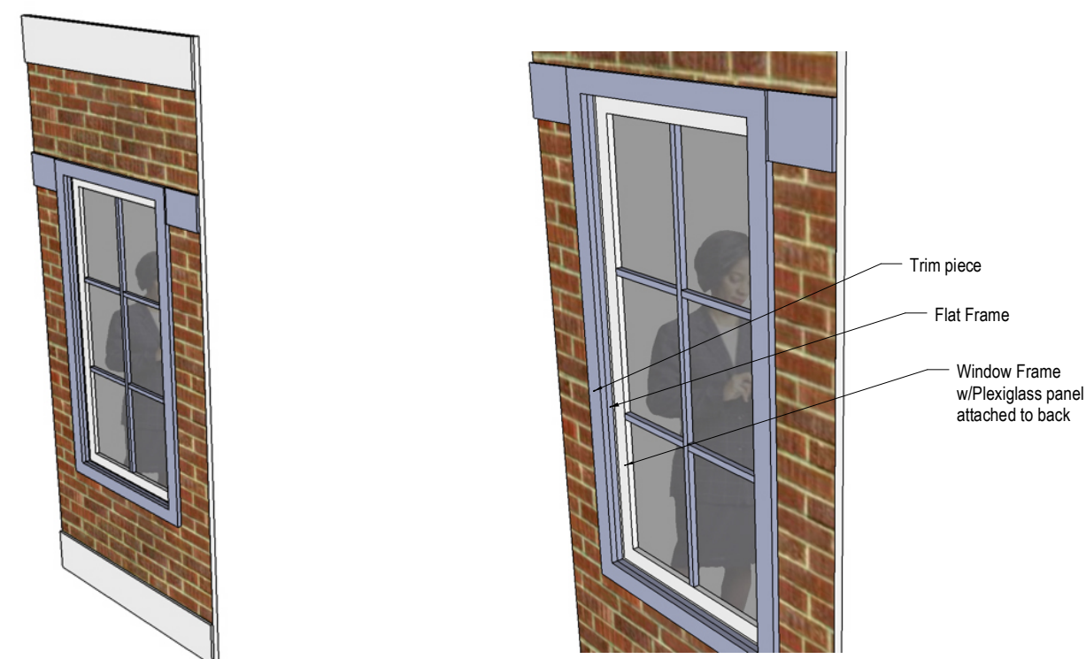
Detail View: Wall B- Typical for Walls A, B, C
