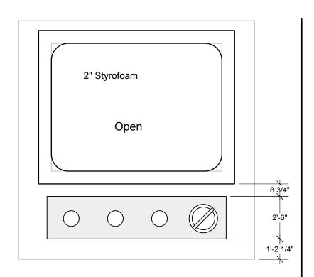
Frame and Controls location on screen face unit (grayed)
