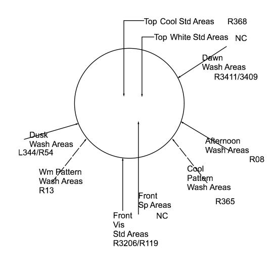
Three Area Systems: **Wash Areas** (A-F), **Standard Areas** (1-11), **Special Areas** (SP2, SP4, SP5, SP6, SP8A, SP8B, SP7, SP9A, SP9B, SP10A, SP10B, SP11A, Sp11B). Special Areas are tightly focused and steeper angle.
